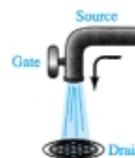
Figure 5.3 Water analogy for the JFET control mechanism.
