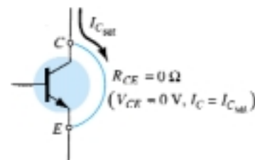
Figure 4.9 Determining I_{C_{sat}} .
