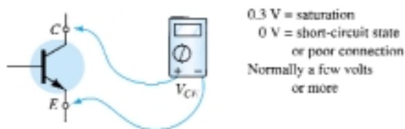
Figure 4.58 Checking the dc level of V_{CE} .
