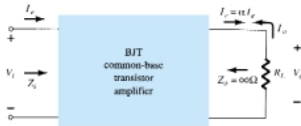
Figure 7.19 Defining A_v = V_o/V_i for the common-base configuration.
